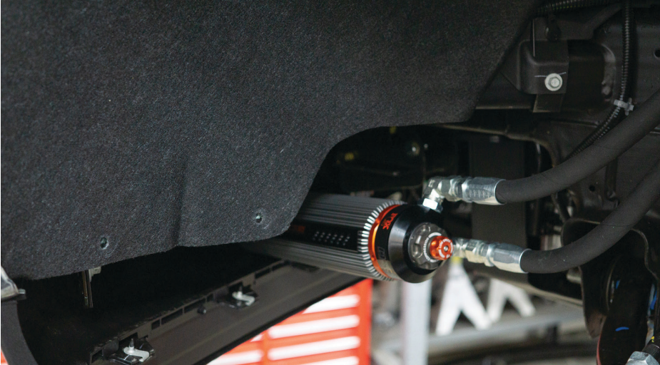
Fig. 23: Cut fender liner.
