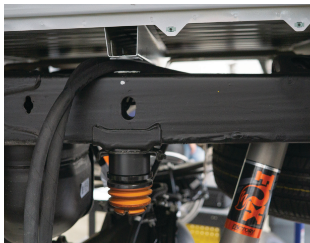
Fig. 34: Pass reservoir between the frame and bed.
