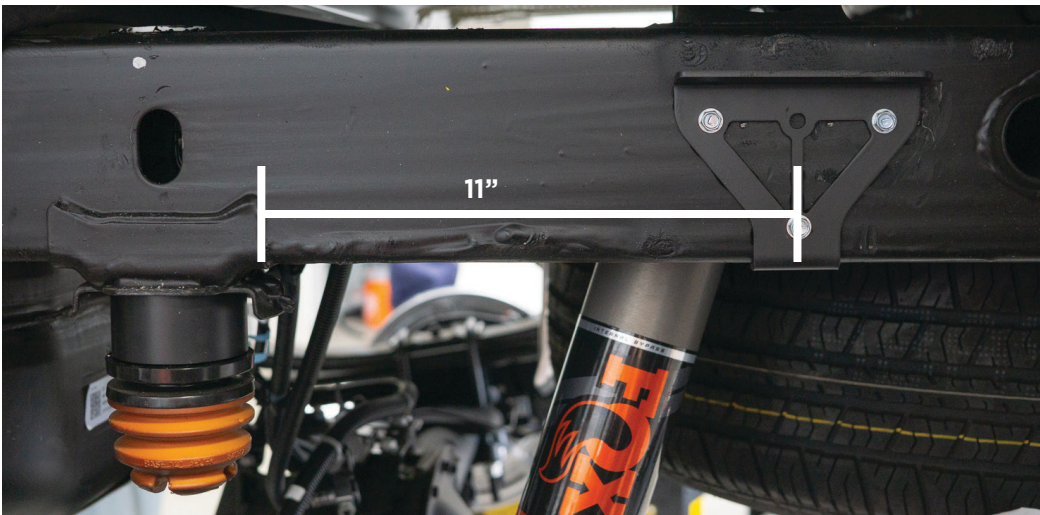
Fig. 37: Mount the reservoir bracket.
