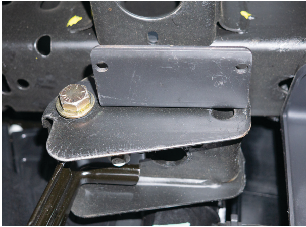
Fig. 11: Use the holes in the vehicles frame.
