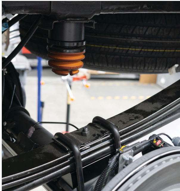
Fig. 26: Install the aftermarket lift block kit.
