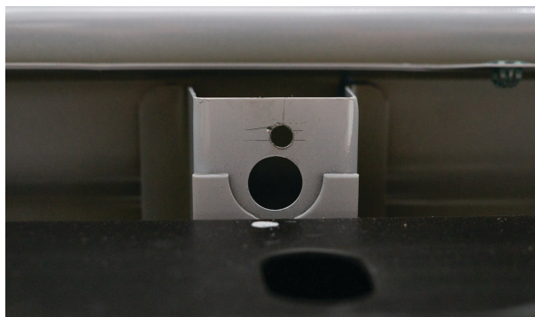
Fig. 29: Center the hole on the frame support.
